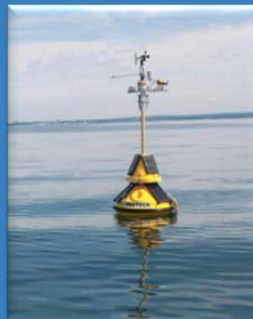
Great Lakes Observing System Hypoxia Warning System buoy deployed north of Cleveland, Ohio. These observations support water managers. Photo credit: Ed Verhamme, LimnoTech
