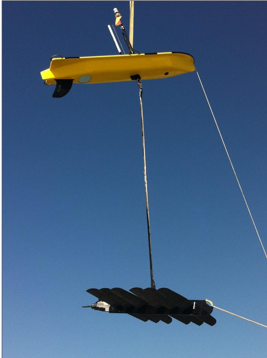
Figure 2-4. Liquid Robotics wave gliders were originally developed for passive acoustic monitoring of marine mammals. (Photo courtesy of Christoph Waldmann/MARUM)
